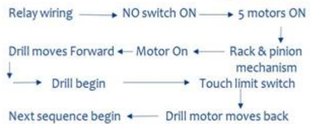
Fig 2: Steps for Sand Core Drilling Automation
