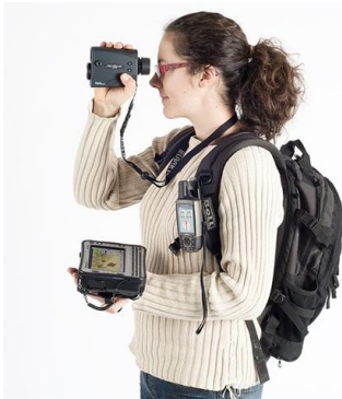
Figure 3 - Example of modern surveying equipment (Field Map technology) GPS, laser rangefinder and computer field allows surveying and mapping (creating real-time map) and field data collection.
