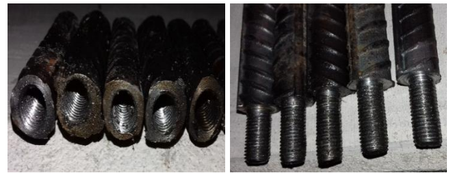
(a) MS tube (b) Threaded rebar
