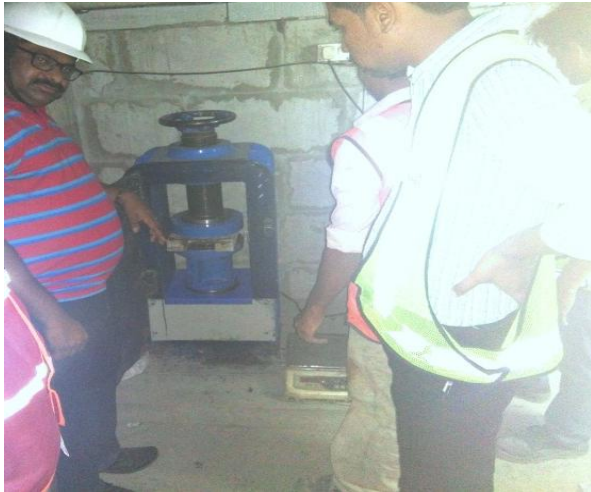
Figure.5 Compressive test carried out on Skin wall Sample.
