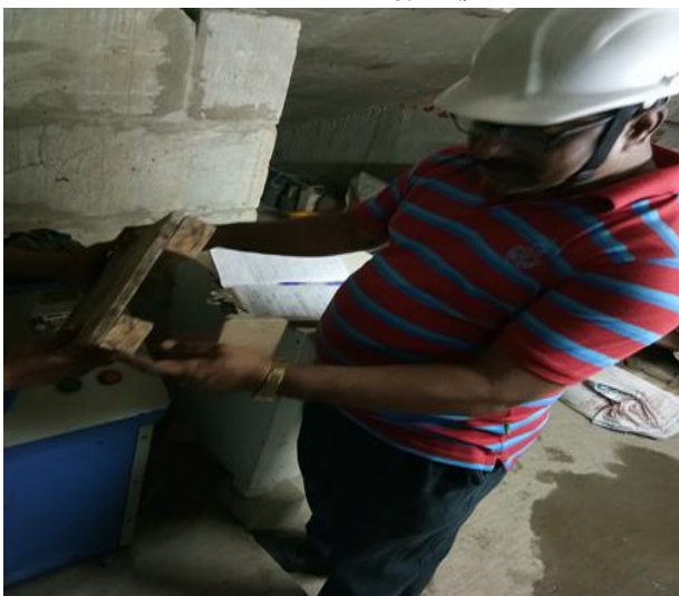
Figure.6 Compressive test carried out on Skin wall Sample
