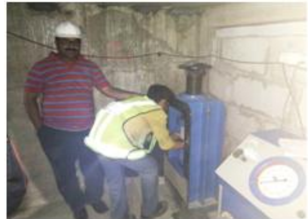
Figure.4 Cube testing of plume concrete wall (M5) for compressive test
