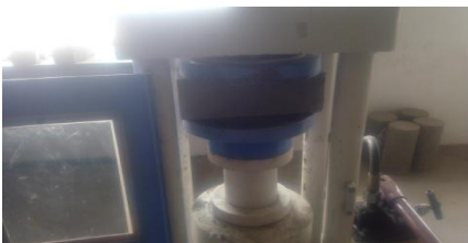
Fig. 13 Crushing strength tested on bricks
