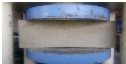
Fig. 14 failure mode of bricks
