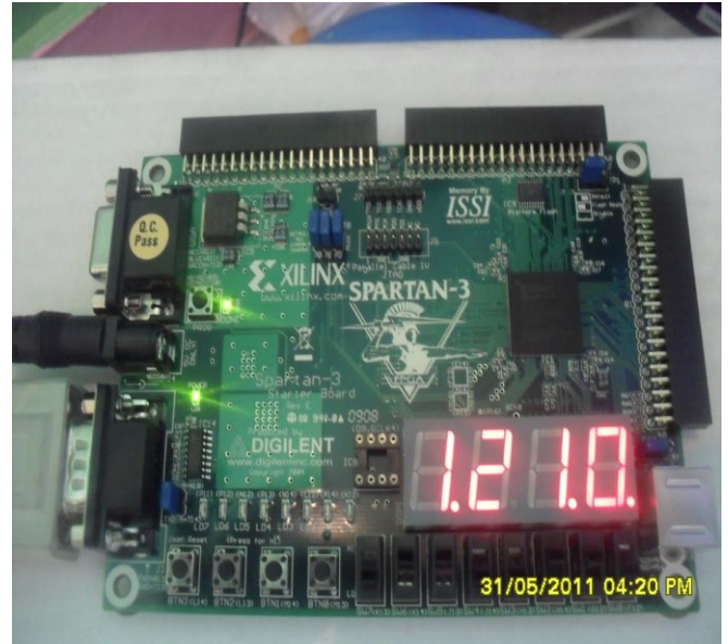
Fig. 10. The alarm is raised when the time is set at 12.10. The indication is the red dots blinking below the digits
