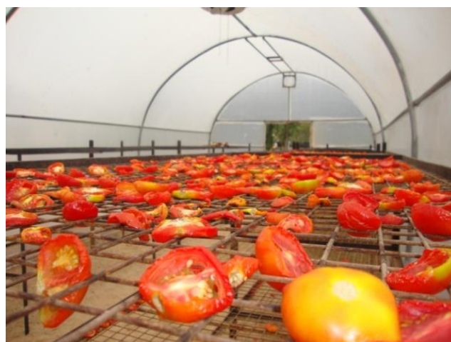
Fig.7 Tomatoes dried inside the solar tunnel dryer
