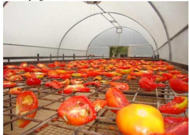
Fig.8 Sliced cut tomatoes dried inside the solar tunnel dryer
