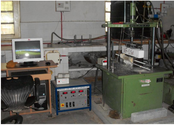
Figure 1 Flexural fatigue test setup
