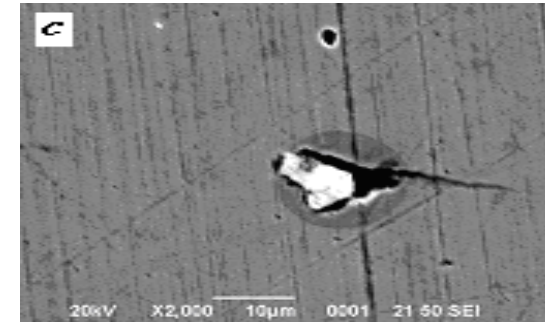
Fig.10 (a) (b) and (c): SEM micrographs showing lead, copper and aluminium transfer layer on ground EN8 steel surfaces (SiC wheel polished). (X2000)
