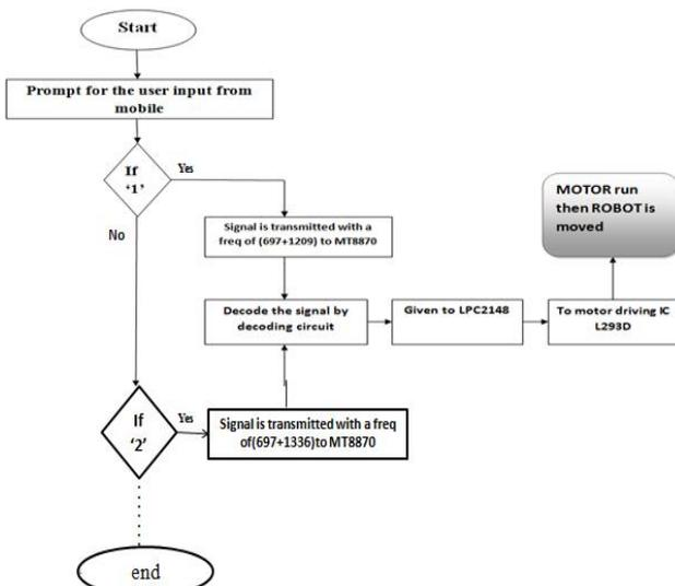
Fig 5: Algorithm for DTMF controlled robot
