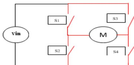
Fig 2: Structure of H-bridge (Highlighted in red color)
