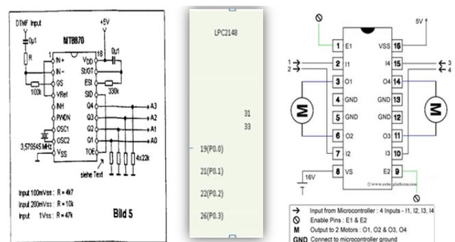
Fig 4: Interfacing of MT8870, LPC2148 and L293D
