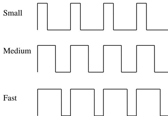
Fig 3: velocity control of motor using PWM
