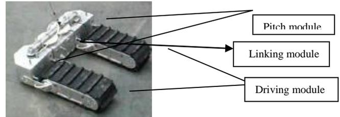
Fig 6: Prototype of climbing robot
