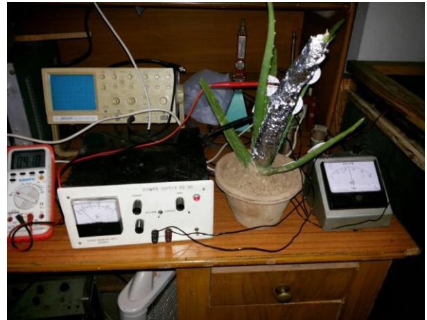
Fig. 6 Setup to calculate resistance of the Aloe Vera leaf.
