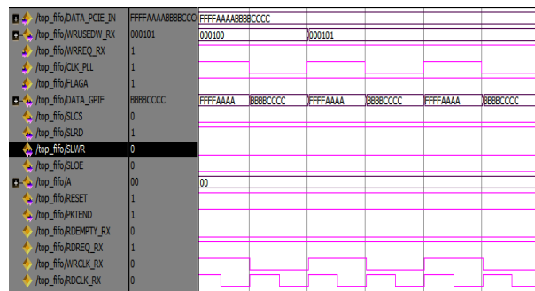
Fig. 9. Simulation result showing data transfer between host controller and device controller
