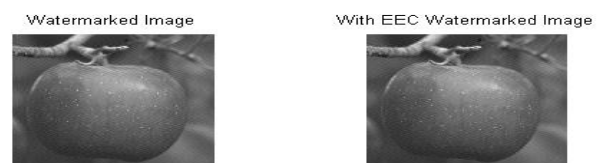
Figure 8(i) Watermarked image with Error Correcting code (Cyclic Code) with PSNR = 54.1896 dB and Compression Ratio = 62.0949%
