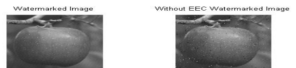
Figure 8(h) Watermark image without Error Correcting code with PSNR = 37.0814 dB and Compression Ratio = 62.0949%
