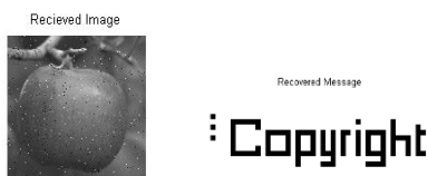
Figure 8(b) Watermark Recovery without attack with PSNR = 23.6388 dB and Compression ratio = 62.0949%
