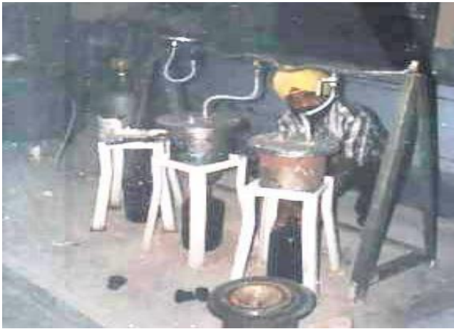
Fig 3: Water Permeability Test Apparatus
