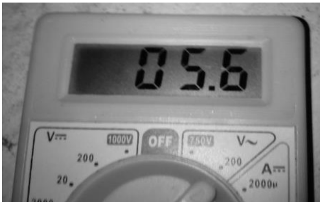
Fig.7 Voltage of 5.6 V Produced at 250 rpm
