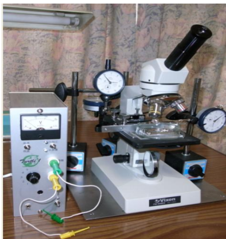
Fig.1. Micro-EDM Set-Up (T.Masuzawa)
