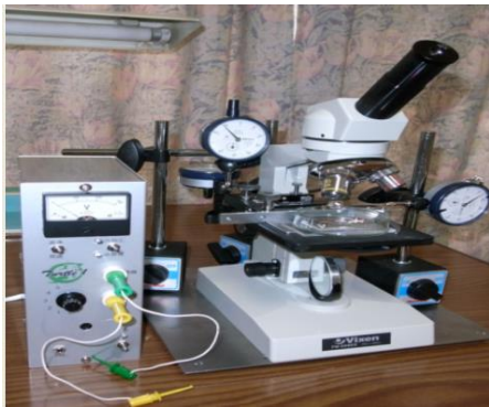
Fig.1. Micro-EDM Set-Up (T.Masuzawa)
