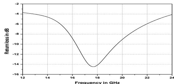
Fig 3: Return loss of the Conventional antenna.
