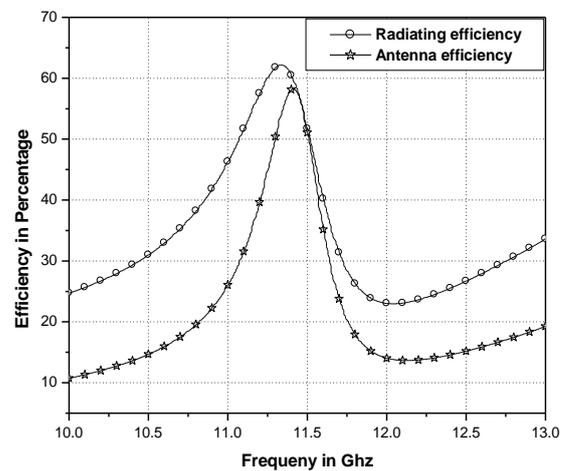
**Fig 8: Antenna efficiency versus frequency plot for the antenna 2.**
