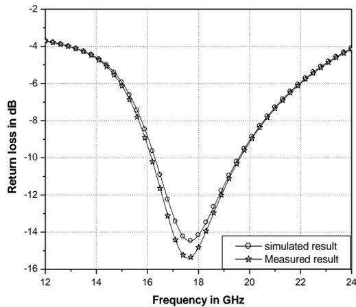
Fig.9. Comparison between measured and simulated return losses for antenna
