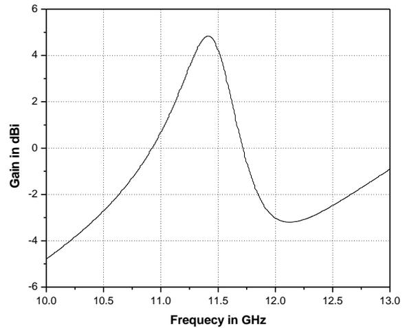
**Fig 7: Gain versus frequency plot for the antenna 2.**
