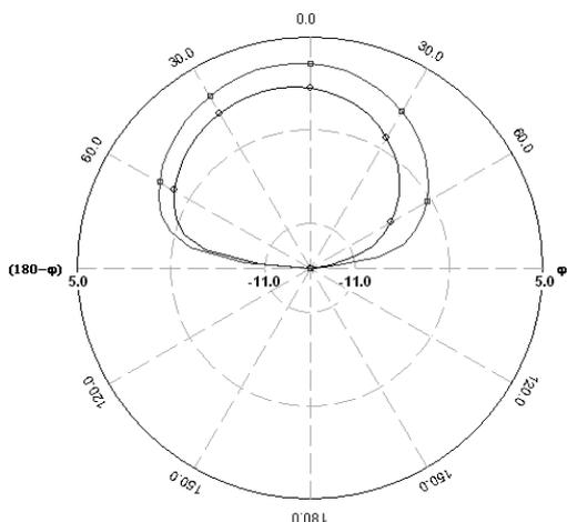
**Fig 6: H plane Radiation Pattern of the antenna 2 for 11.4 GHz**
