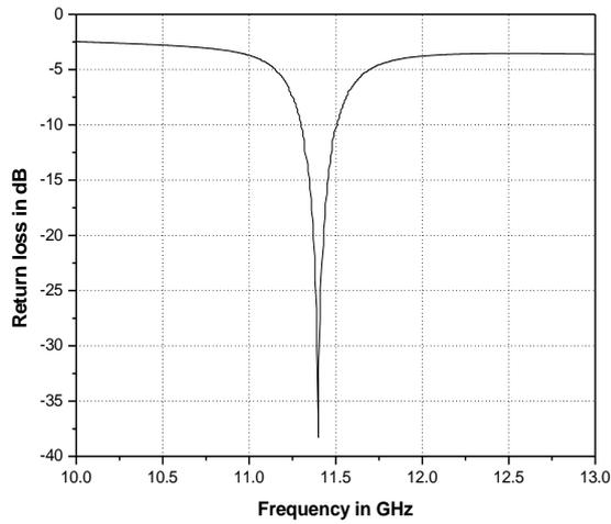
**Fig 4: Return loss of the proposed antenna.**
