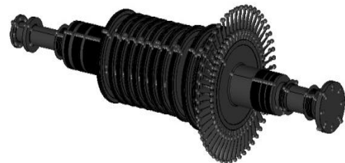
Fig 01: shows the CATIA model of rotor and blades of a LP impulse-reaction turbine
