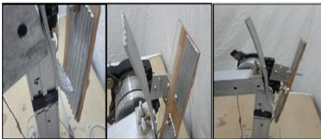
Figure 13 Limit Switch down side Figure 14 Limit Switch up side Figure 15 Side View of Limit Switches
