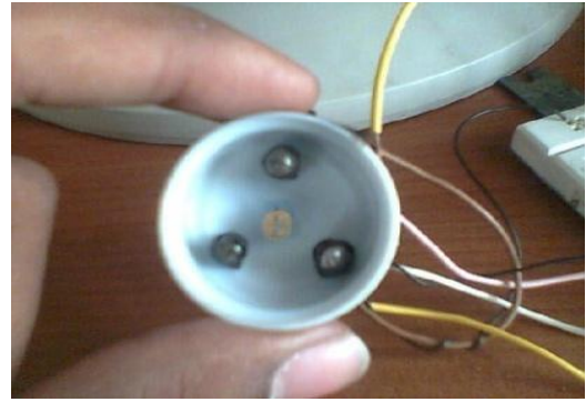
Fig. 8 Sensor unit design to measure pH level
