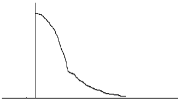
Fig. 14 General Response of Amplitude Butterworth Filters
