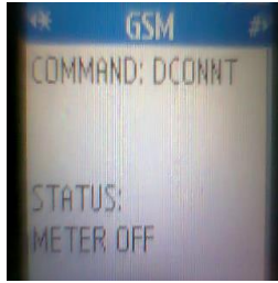
Fig.9: By sending the command “#DCONNT” through the mobile phone the GSM modem receives the command and the load will be disconnected and an reply message will be sent to the mobile phone regarding the current status of the system.
