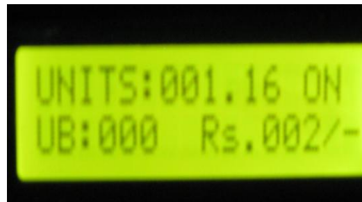
Fig 7. LCD showing the energy consumption values, billed amount and status of the system is also displayed when system is ON.
