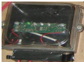
Fig 4. ADE 7757 Energy meter
