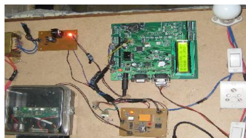
Fig 8. Wireless meter reading PCB when the Load is OFF and the interfacing of Energy meter, ARM7 (LPC 2148) Microcontroller modules.
