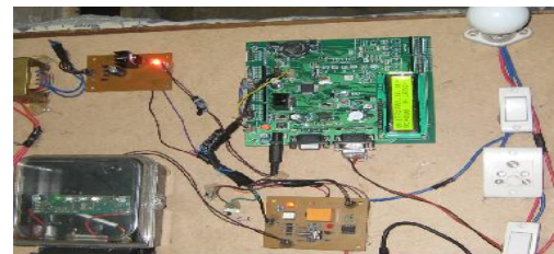
Fig 8. Wireless meter reading PCB when the Load is OFF and the interfacing of Energy meter, ARM7 (LPC 2148) Microcontroller modules.
