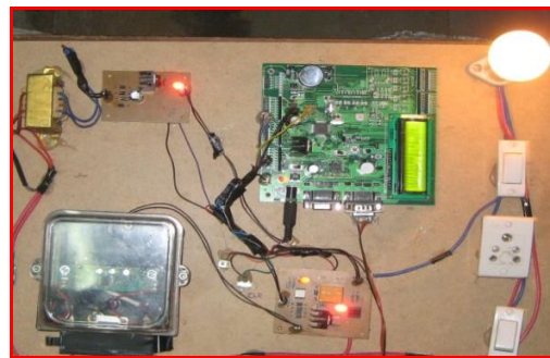
Fig 6. Wireless meter reading system PCB when the load is ON and the interfacing of Energy meter, ARM7 (LPC 2148) Microcontroller modules.
