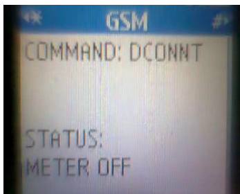
Fig.9: By sending the command “#DCONNT” through the mobile phone the GSM modem receives the command and the load will be disconnected and an reply message will be sent to the mobile phone regarding the current status of the system.
