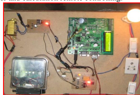
Fig 6. Wireless meter reading system PCB when the load is ON and the interfacing of Energy meter, ARM7 (LPC 2148) Microcontroller modules.
