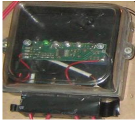
Fig 4. ADE 7757 Energy meter
