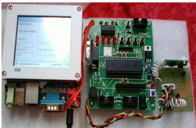
Fig. 5 ARM 920T S3C2440 processor with Sensor expansion board
