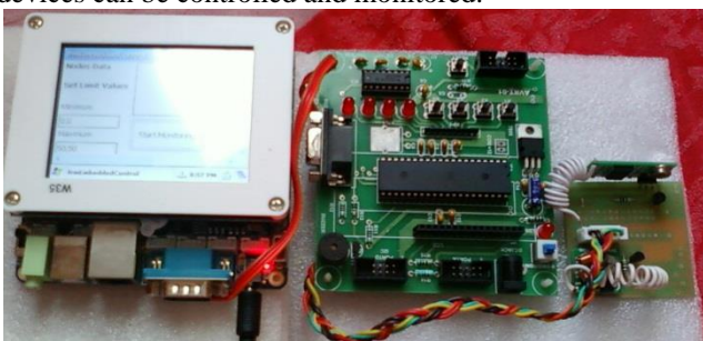
Fig. 5 ARM 920T S3C2440 processor with Sensor expansion board
