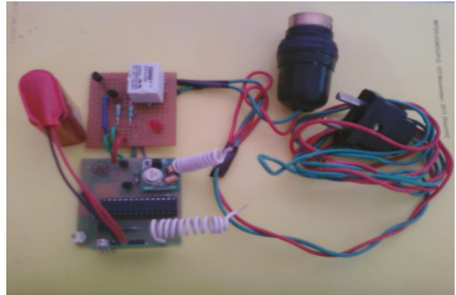
Figure 6. represents the hardware implementation of wireless sensor node .Each wireless sensor node attached with electrical device via relay.
