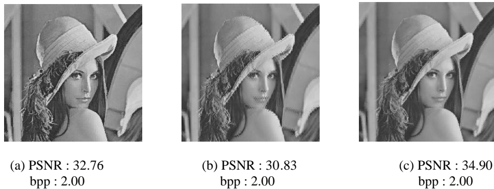
Figure 2. Comparison of the reconstructed images using existing (a) BTC, (b) BTC Variant and (c) AMBTC methods
