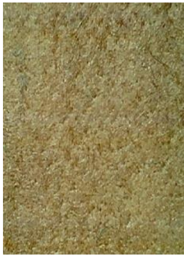
Fig. 6(b): Jute Felt of 12mm thick and GSM 1650
