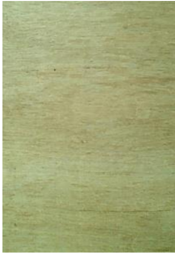
Fig. 6 (a) : Plywood with Gurjan as face veneer
