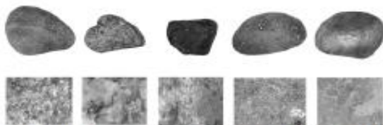
Fig. 6. Top row shows the five rock images out of 60 rock samples used for the experiment. The bottom row shows grain images of corresponding rocks with magnification 50x. For each rock six grain samples are collected one of each grain sample shown here.
