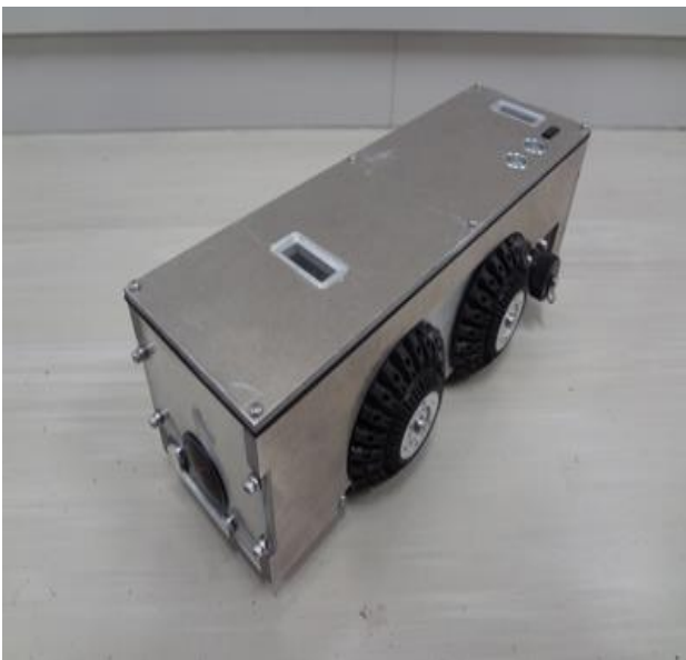
Fig. 1: Target Piping Inspection Robot
