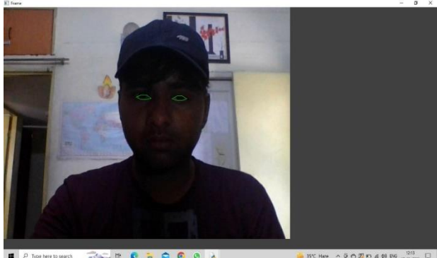
Fig 2: A photo of the driver is uploaded, and eyes are identified by the system.
