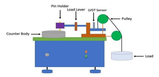
Fig. 6. Tribometer experimental set-up.
