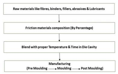
Fig.4. Brake pad fabrication process.
