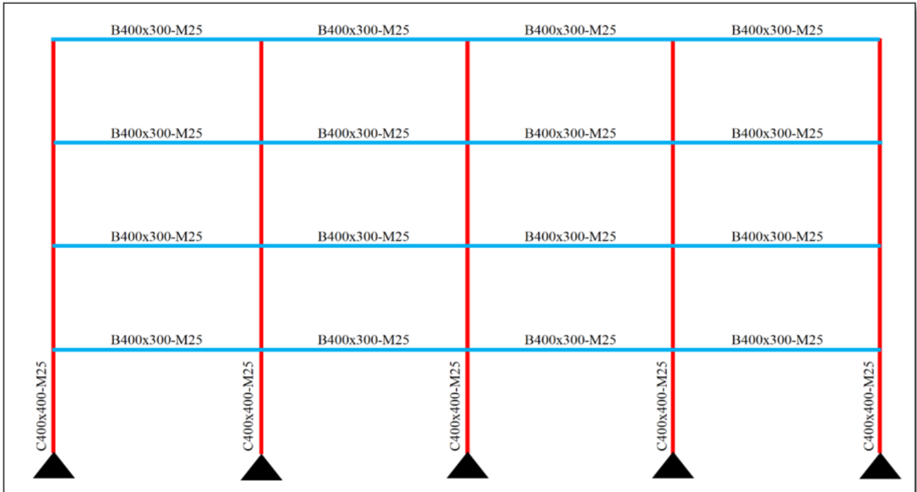
Figure 10. RCC Frame Structure Section Properties
