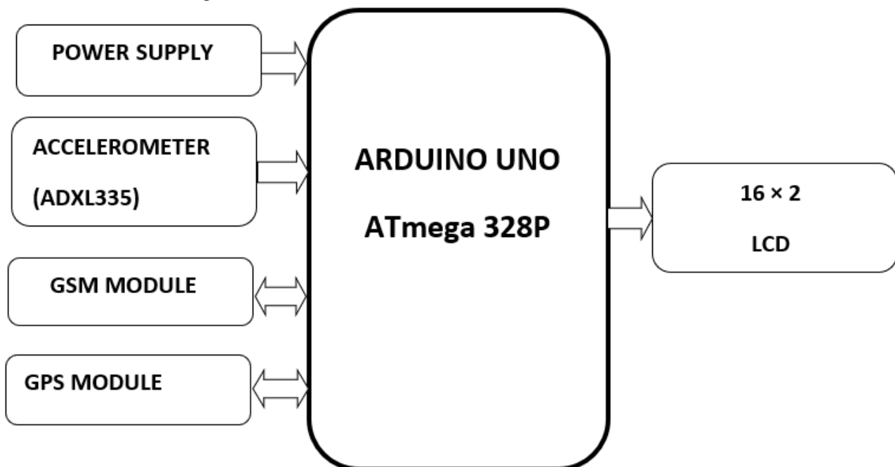
Fig 1: Block Diagram of the Accident Detection System
