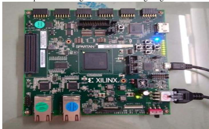
Figure 11: Implementation of ALU with SP701 FPGA Board
