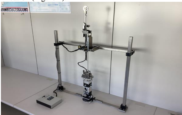
Fig. 2 Appearance of Contact Type Three-Dimensional Position Measuring Instrument
