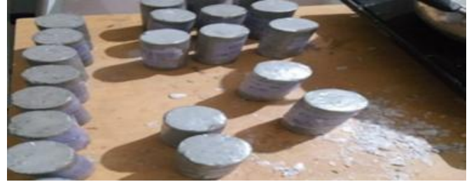
Fig 1. Wax coated stabilized Pond ash samples prepared for curing in humidity chamber
