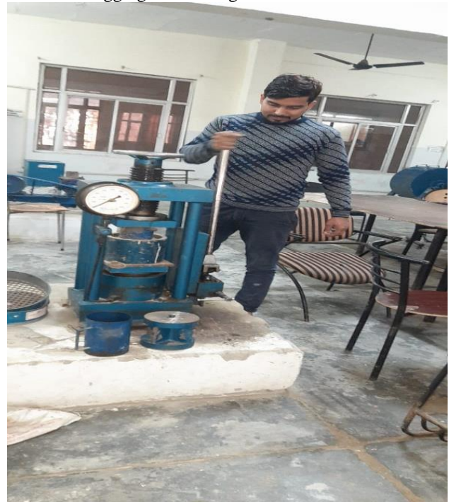
Figure 4. Crushing value test
