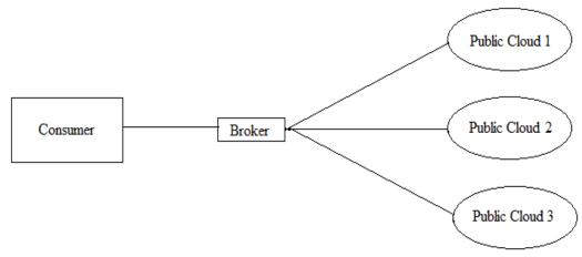
Fig.3. Cloud Broker Architecture [20]
