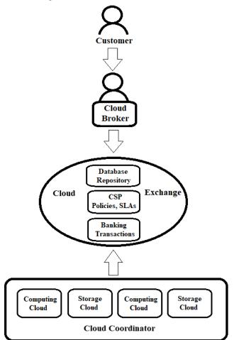
Fig.1. Federated Cloud Architecture
