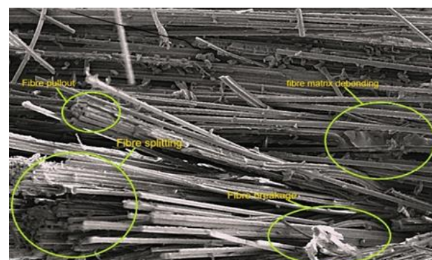
Figure 15.b) SEM image of air bubbles, fiber breakage and matrix debonding of flexural specimen
