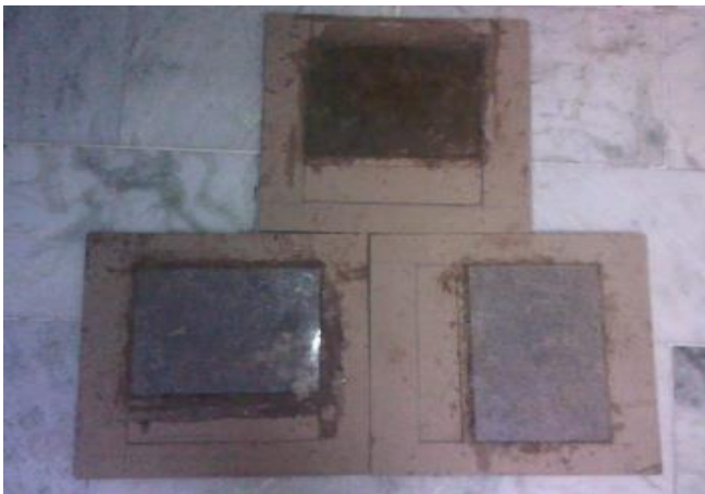
Figure 3 Compression moulding technique of hybrid composite specimen
